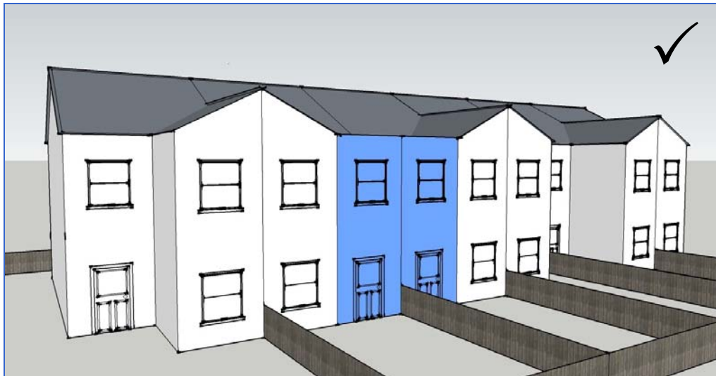
Figure 5 Two storey rear extensions built simultaneously to adjoining terraces
