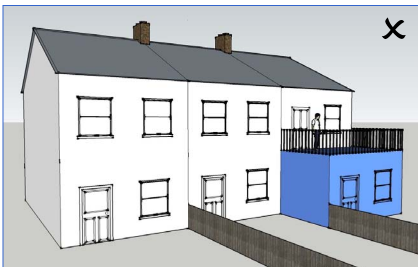
Figure 4 Single storey rear extension with balcony causing overlooking
