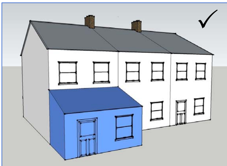
Figure 3 Single storey rear extension with pitched roof
