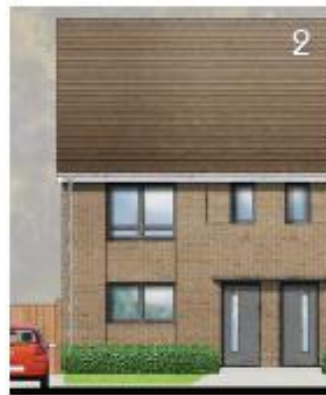
2 Recessed brick panel alongside upper floor windows
