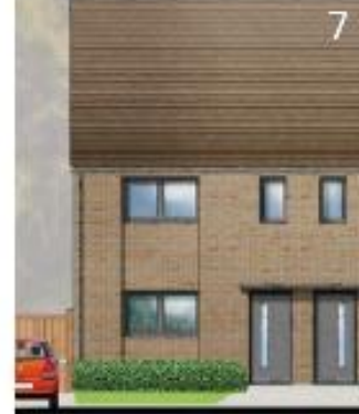
7 Final elevational design and materials proposals: incorporating the materials alterations (1), clipped verges and rise and fall gutter brackets (4), and a solid roofed cantilevered porch
