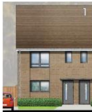
1 Material changes: brown brick and earthy-toned roof tiles, recessed brick panels between windows in same brick, front doors in grey
