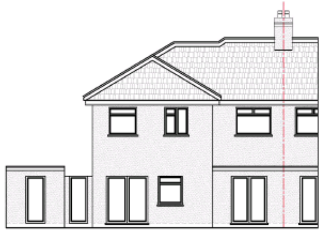
EXISTING REAR ELEVATION SCALE 1:100
