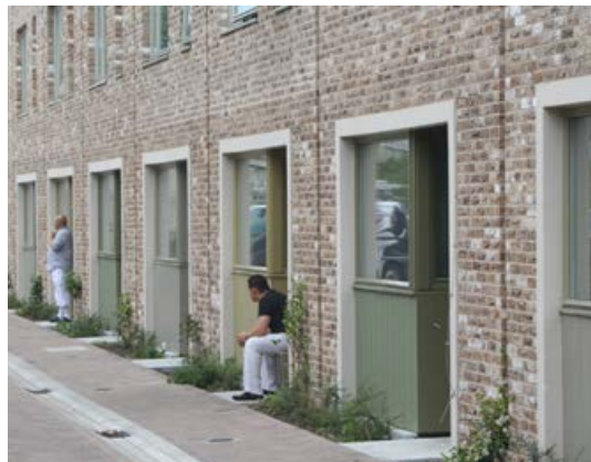
Planting strips outside dwellings in home zones allow residents to personalise their entrance while keeping a uniform street scene (Barking town centre)
